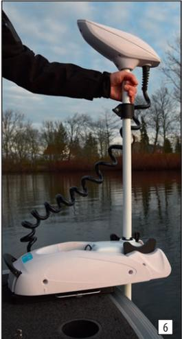
Hold the motor shaft with one hand, then loosen the depth adjustment screw and set the motor to the desired depth. Engage the depth adjustment in the steering unit (Fig. 6) and then tighten. Then align the motor head if necessary.
