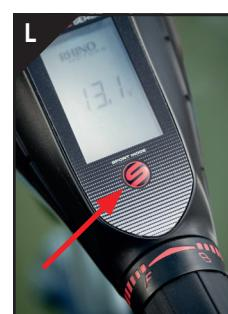
2. Turn the handle clockwise to maximum position, Then press the S button again.
